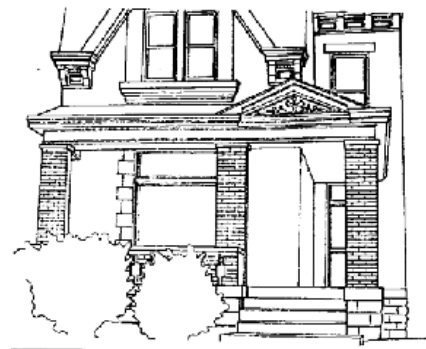
Example of a late Victorian period residence with added Bungalow style brick piers.
