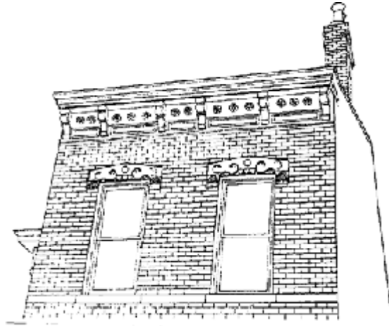
Example of sheet metal cornice design common in the district.
