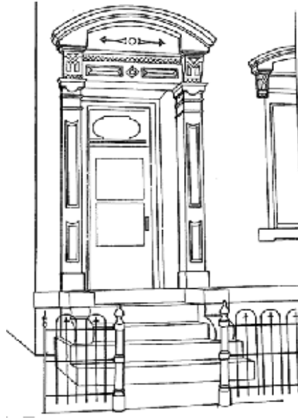
Example of an original Italianate door surround.
